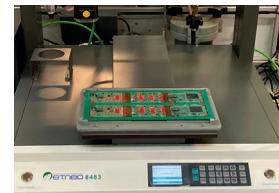
High speed Jet valve dispensing system - Valves and system available
