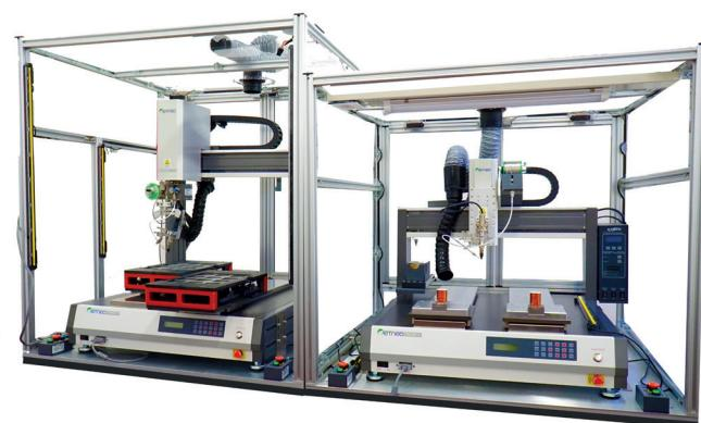
Desktop 2 Y axis + 3 axis with safety box and light optical curtains
