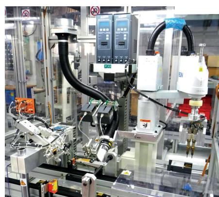
Etneo Soldering parts - Iron unit - wire dispenser - Temperature and parameter real time controller - device for cleaning and aligning the tip, installed ona Scara type robot.
